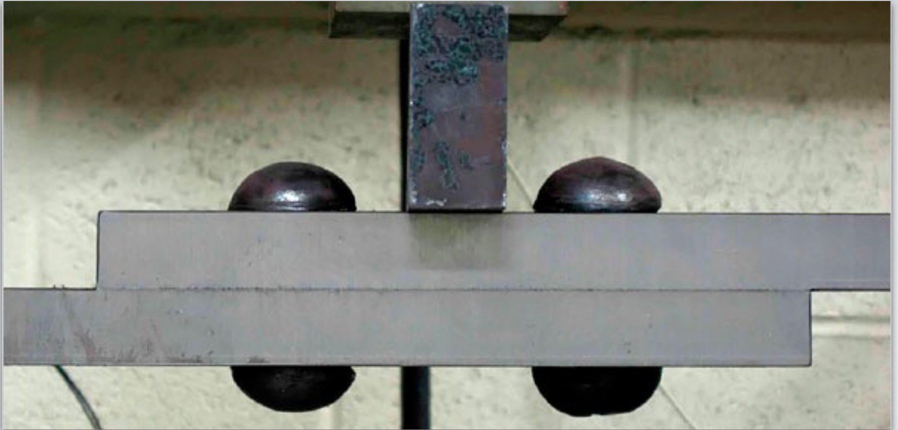
Rivets Holding Overlapping Steel Plates
