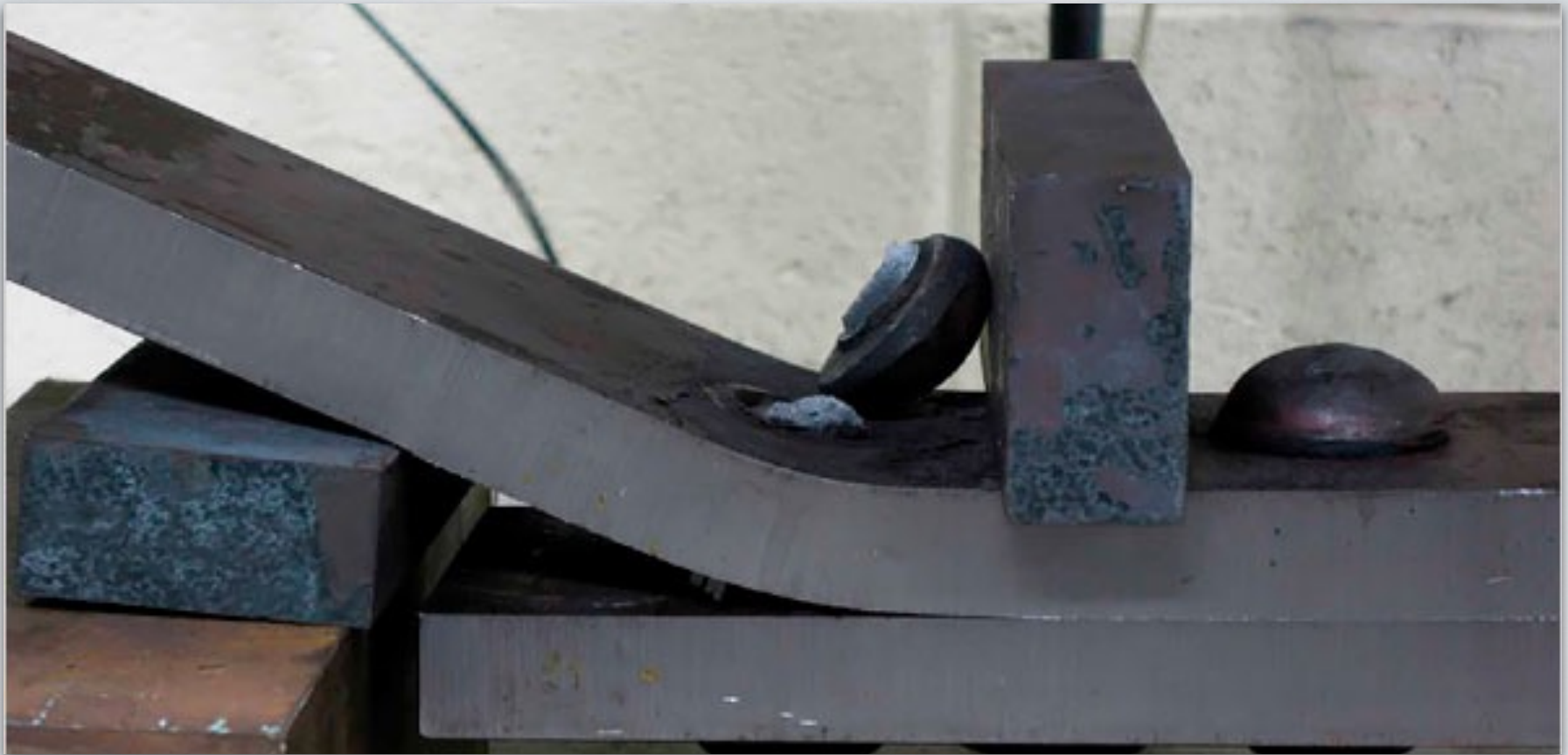
Rivet Head "Popping" After Stress
